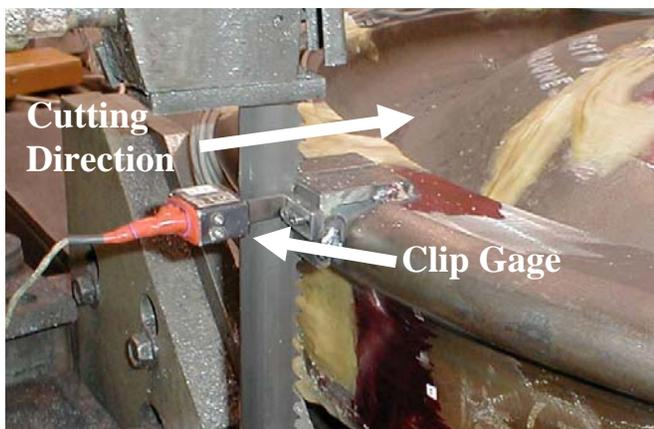
Figure 5. Photo of a Saw Cut Test
