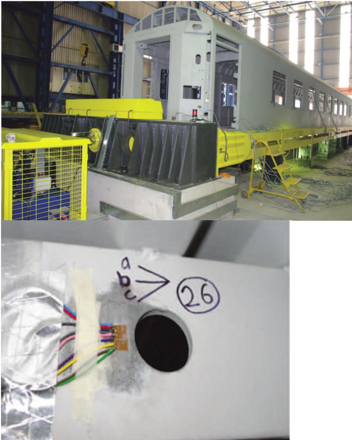
Figure 3 : Experimental Car Test Setup and a Sample Strain Gauge Application
