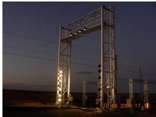
**Figure 12. Fully Automated Train Scanning System installed at TTCI's FAST Facility**
