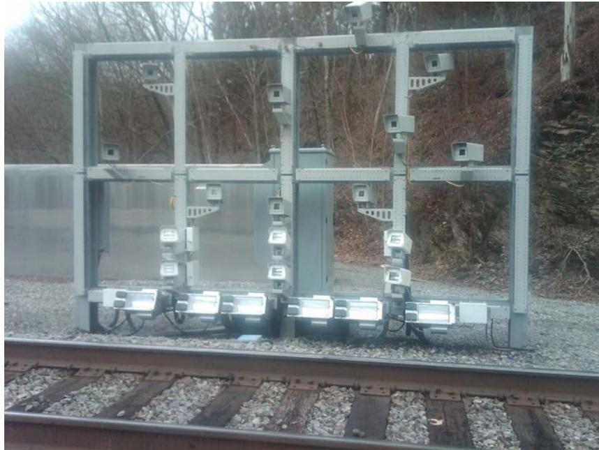
**Figure 3. Beenavision Automated Safety Appliance System on a North American Railway**
