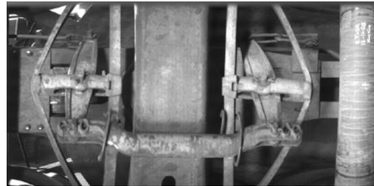
**Fig 9. Truck Bolster and Brake Rigging**
