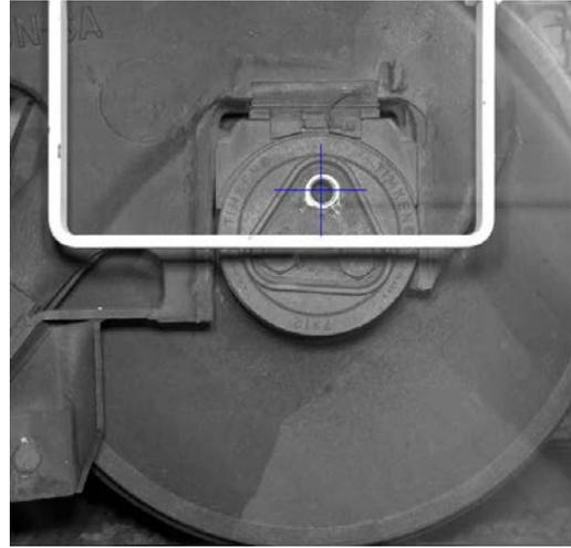
**Figure 7** Spring condition, load balance, wedge condition, end cap bolts, and bearing adapters are diagnosed.
